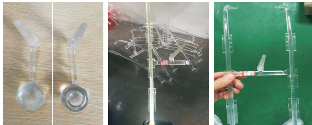
LED透镜COC (普通三机一体) 黄变 LED lens COC (general 3 in 1 machine) yellowing
