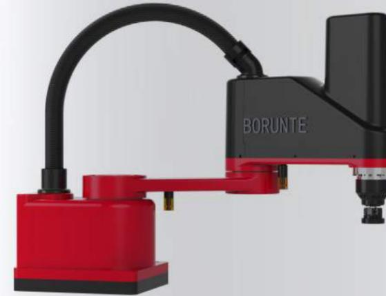
BRTIRSC0603A type robot is a four axis robot that developed for some monotonous, frequent and repetitive long-term operations.The maximum arm length is 600mm. The maximum load is 3KG. Suitable for printing and packaging, metal processing, textile home furnishing, electronic equipment, and other fields . The protection grade reaches IP54 The repeat positioning accuracy is 0.02mm.
