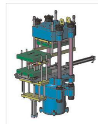
移模单层顶出 Sliding & Single-layer Ejecting
